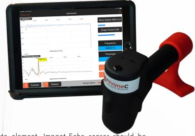
The Steel ball impactor is used to strike the plate element. Impact-Echo sensor should be placed close to the source of impact. Followed by the mechanical impact, reflections are recorded using Impact-Echo sensor. Data are digitized and transmitted to the tablet for post processing, thickness measurement and generating contour plots of thickness variation. Test results are often presented and analyzed in Frequency Domain.
